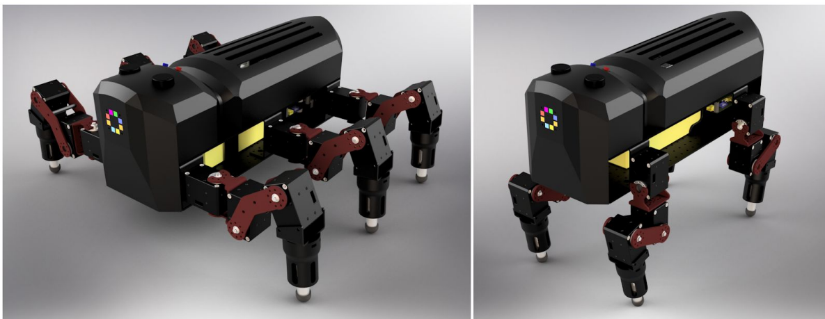
Fig. 1 MORF when configured as an insect and a mammal. When configured as an insect MORF is 38cm wide, 40cm long, and 17cm tall.
